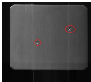
Shortwave infrared solar wafer defect detection
